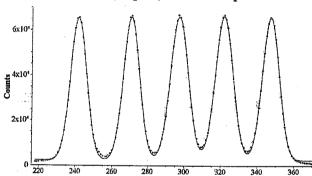
scintillators coupled XP-2020Q photomultipliers. The five coincidence spectra were recorded individually 0.40 m each one apart from the other, with both the scintillators touching the emmiting source in the first position measurement, and with the DET1 remaining in this configuration for all the measurements. The difference between both extreme spectra's fitted centers channels, corresponding to 1.40 m. was estimated 347.34609370 ch 241.70179056 ch= 105.64430314 ch; taking into account the time
