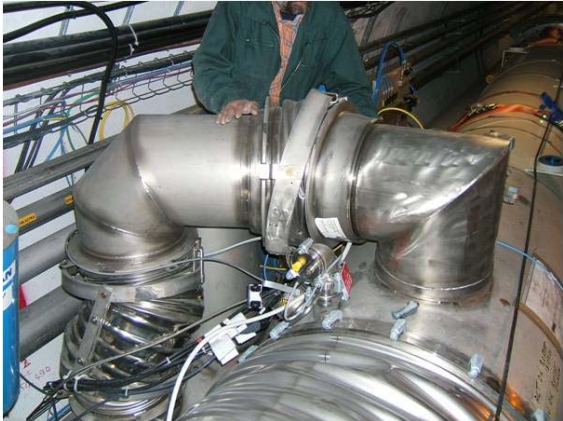
Figure 17: Damage to “jumper” connections of cryogenic distribution line
