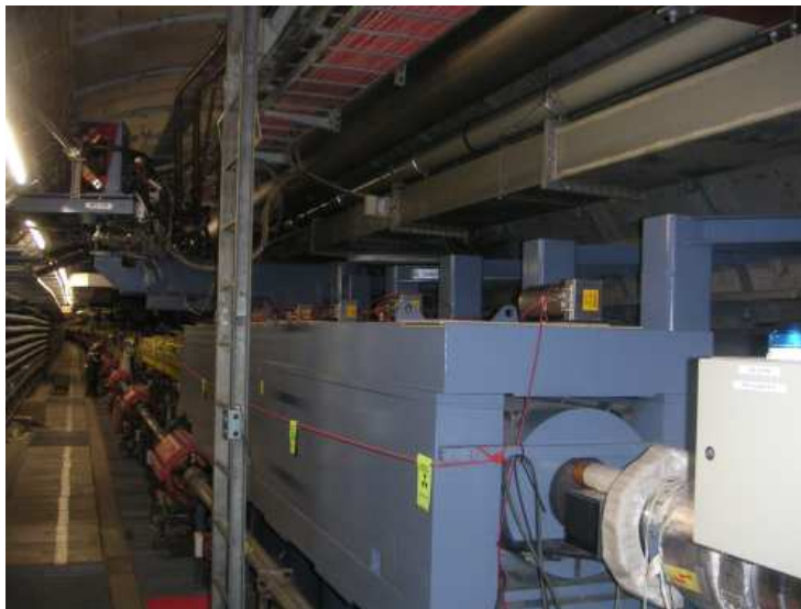
Figure 6.3: Detector installation on the HERA proton beam dump.
