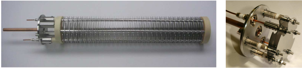
Fig. 4.2.: Inner structure of an IC (left) and inner structure of a SEM (right).
