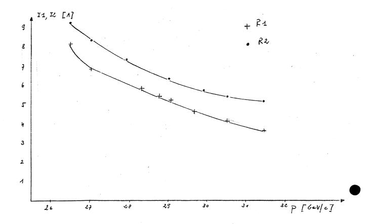
Fig. 1 Current losses in R1 and R2 during accelevation
