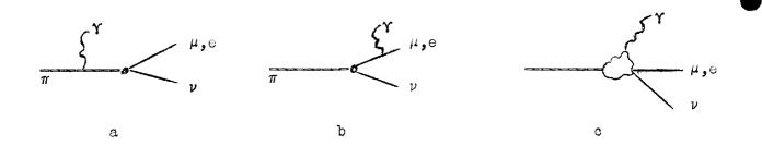
The inner bremsstrahlung contribution can be computed in a straightforward way, while the two direct contributions are very interesting. The vector contribution is related by CVC to the  $\pi^0 \to 2\gamma$  decay. Its determination would then constitute a new and independent test of one of the cornerstones of the
