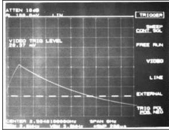
Figure 3.4: Time domain signal from HOM pickup on the 2585 MHz mode.
