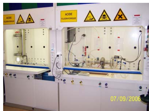
Figure 1: Electro-polishing set-up at CEA Saclay.
