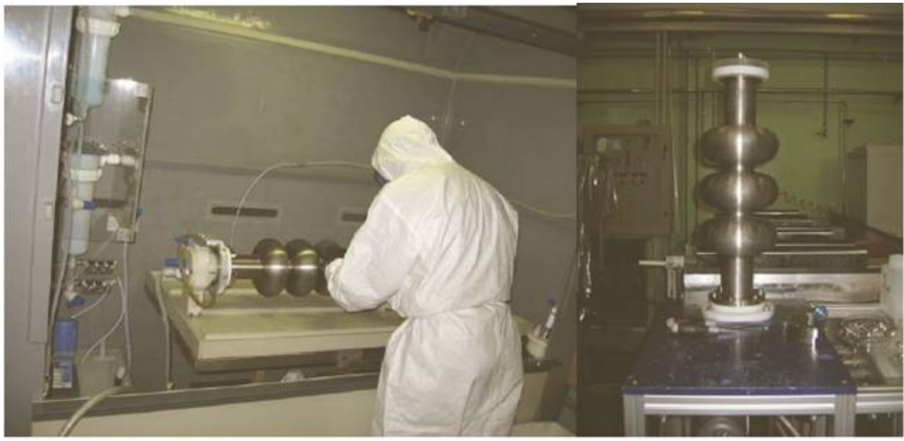
The 3-cell cavity was then titanified and it is ready for rf measurement.
