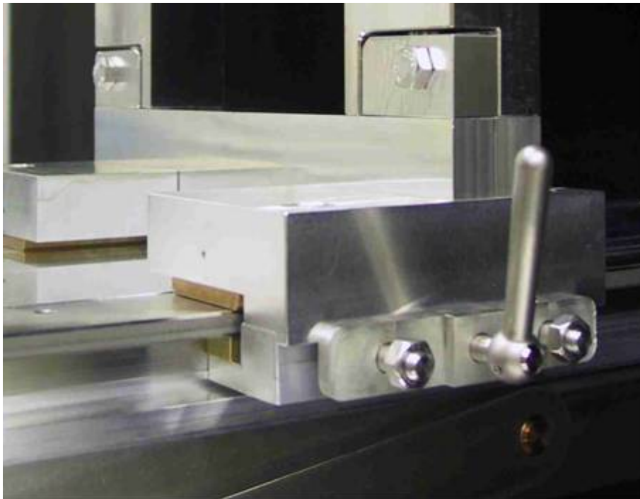
Figure 2: To change the working-position of the support, we use a quick release fastener
