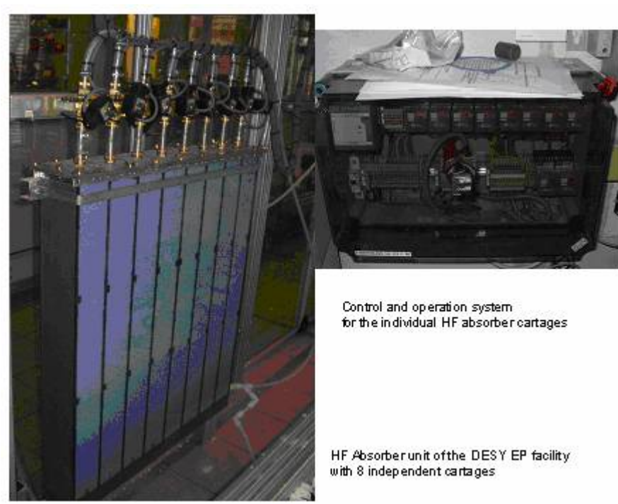
Pic 9 Picture of the new development of gas scrubber for HF exhausting gasses
