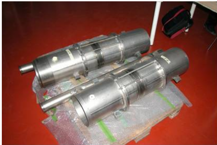
Figure 3: TTF cavities modified helium tanks
