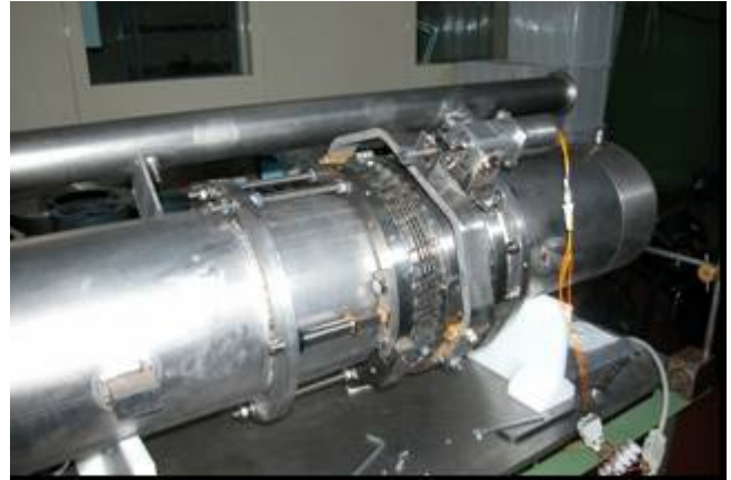
Figure 5: Complete assembly provided with leverage mechanism and stepping motor.
