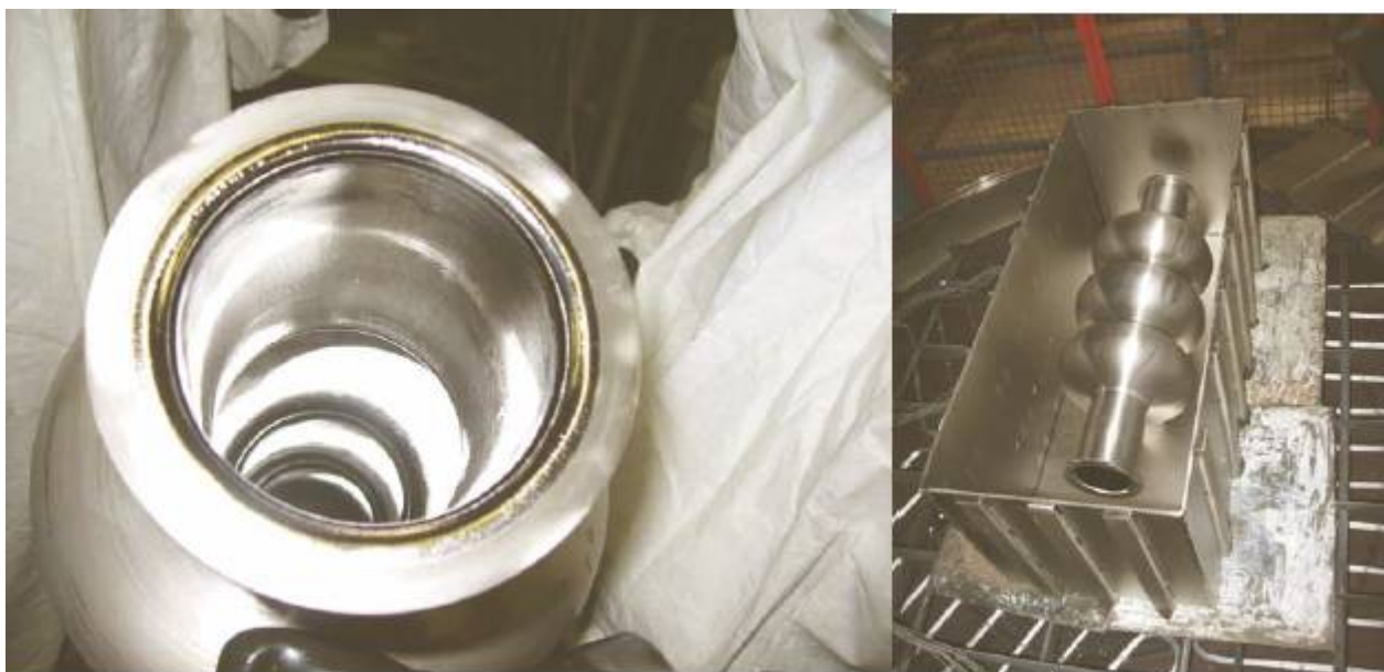
The first 3-cell prototype has an innovative flange design that has been fabricated seamless without the need of EB welding
