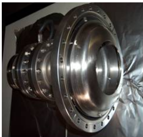
Fig.2. Picture of the new collector system, as taken before its assembling on the UHV stand.
