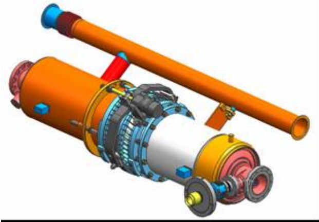
Figure 4: The cavity dressed with the modified helium tank and piezo blade tuner.
