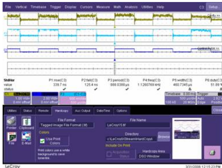
Fig.6. Time variations of the ion current, as collected by the “cavity” wall during the application of pulsed bias voltage. The upper trace shows the current readout, the second trace presents a
