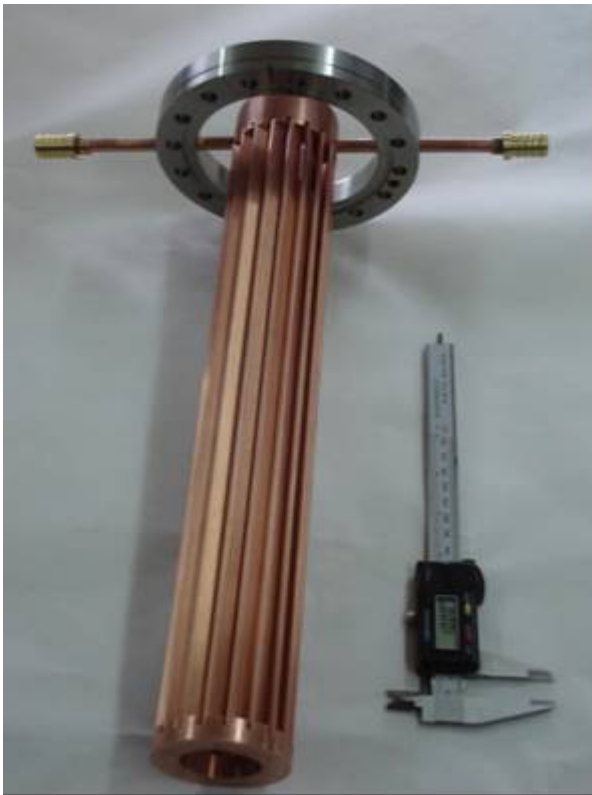
Fig. 1. General view of the cylindrical Venetian-type micro-droplet filter.
