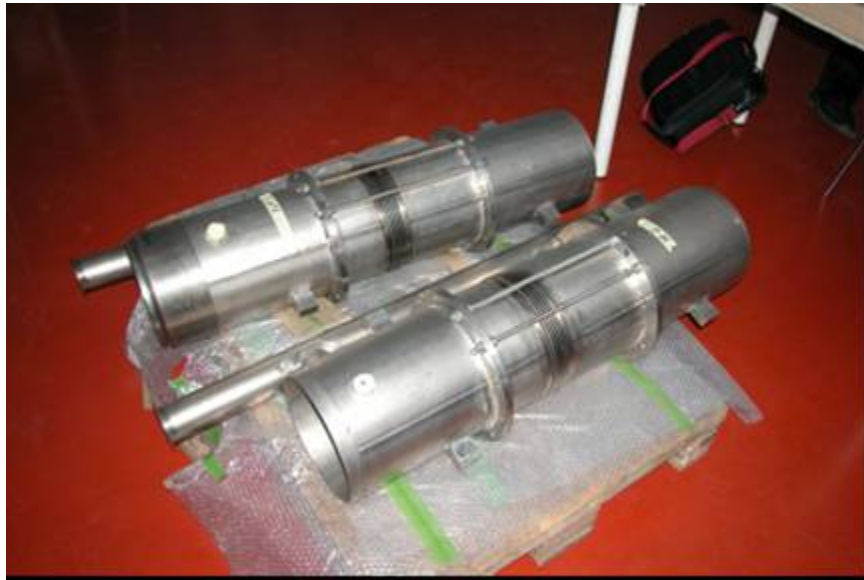
Figure 4: TTF cavities modified helium tanks
