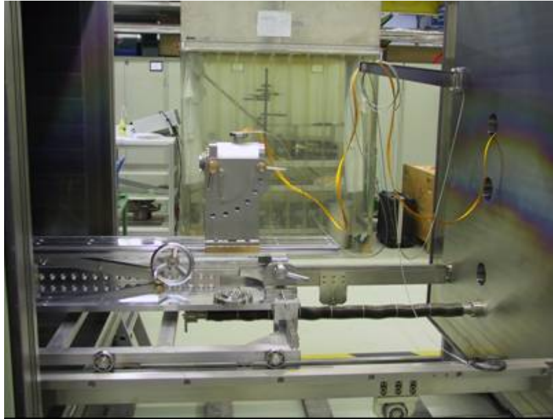
Figure 1: motor box and current supply with Kapton© isolation
