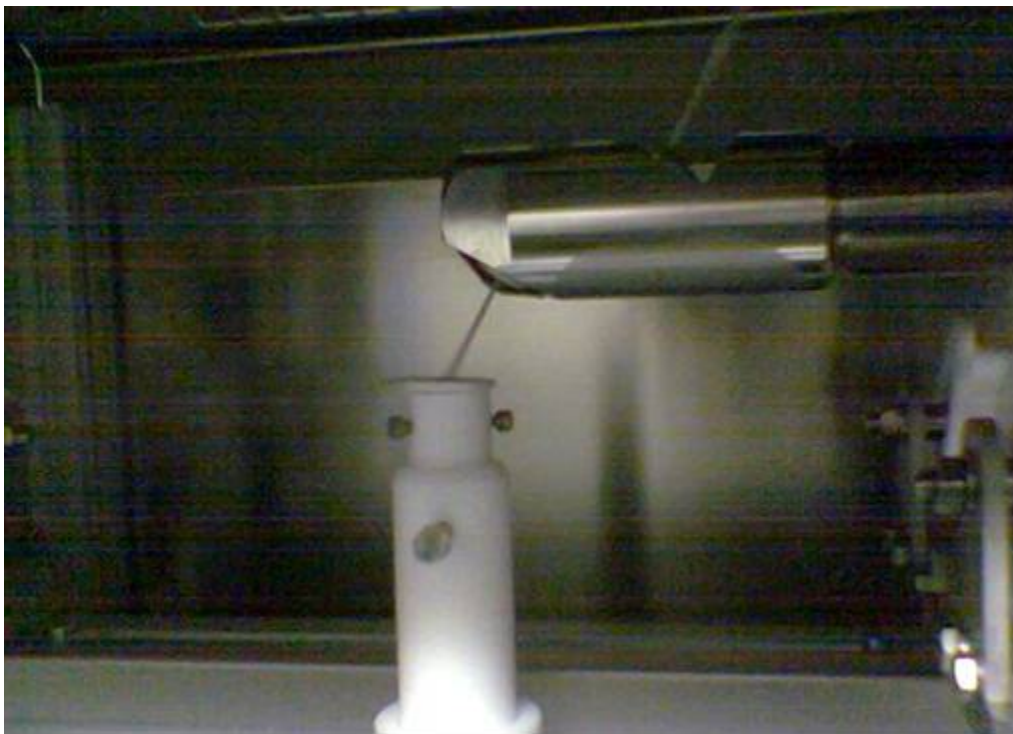
Cleaning of a niobium sample for field emission investigations (WP6.3)
