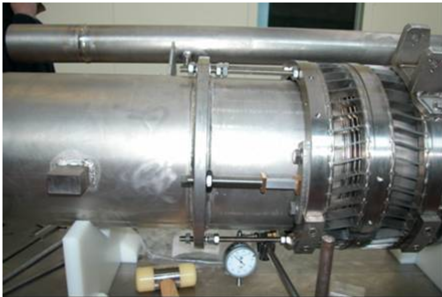
Figure 6: Dummy piezostack block inserted in the coaxial tuner
