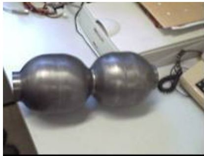
Fig. 3: Example of the Nb tube necking
