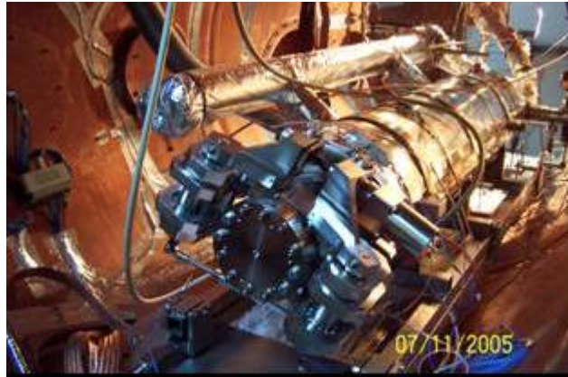
Fig.4 Cold Tuning System (CTS) with Noliac or PICMA Piezoelectric Tuners mounted on 9-cell C45 cavity in CryHoLab.
