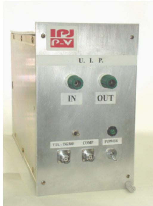
Fig. 5. General view of the U.I.P Keying Module used for pulse biasing of RF cavities.
