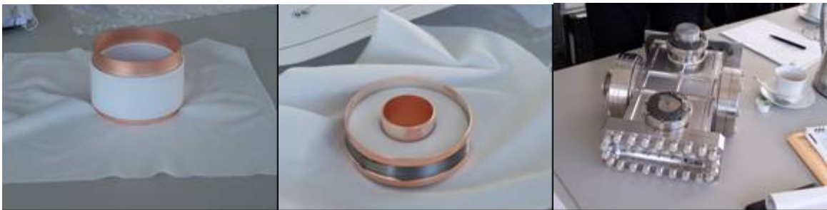
From left to right: TTF5 brazed production ceramic, TW60 validation ceramic, test transition
