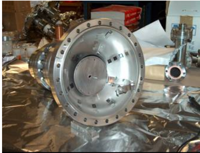
Fig. 5. View of the ion current collectors installed inside the upper half-cell.
