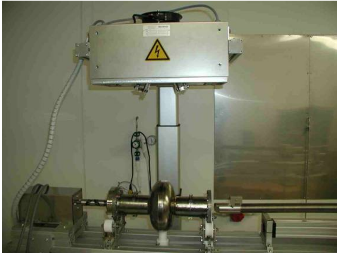
Dry-ice cleaning system with the new IR heater
