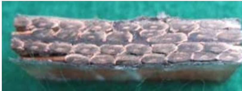
Figure 12: Sample after shear testing. Note how poor the bond appears between the insulation and cable
