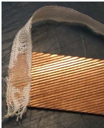
Figure 8 a & b: Wrapping of Atlas Cable with tape
