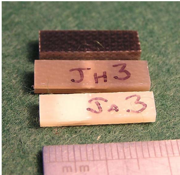
Figure 1 Illustrating contamination due to carbon residue from sizing decomposition. The laminates are short-beam-shear samples, after testing.
