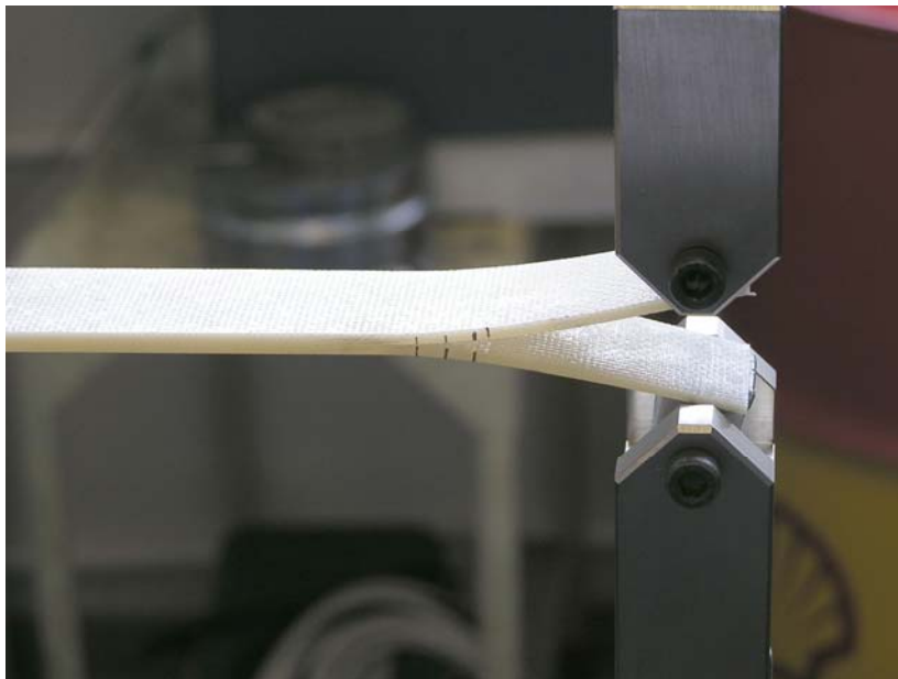
Figure 3 Interlaminar fracture testing to ASTM5528 of a non-heat treated laminate
