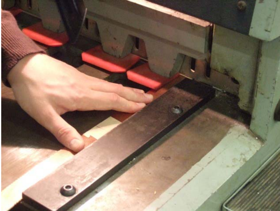
Figure 6: Cutting of ATLAS cable using a guillotine
