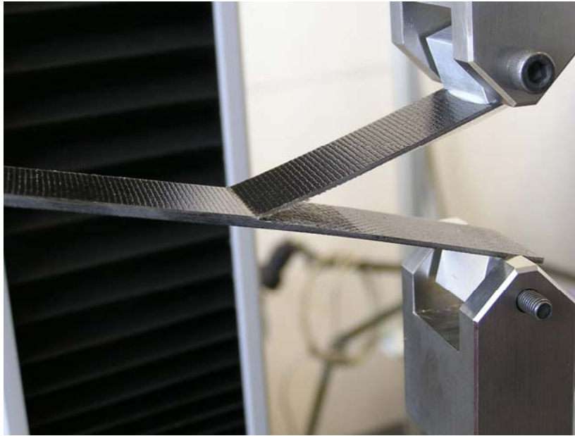
Figure 4 Interlaminar fracture test of a laminate contaminated with carbon from sizing decomposition, note the black colour and crack propagating through the glass fibre.
