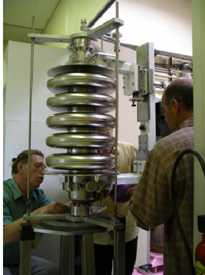
Figure 51: The cavity under assembly in Saclay.
