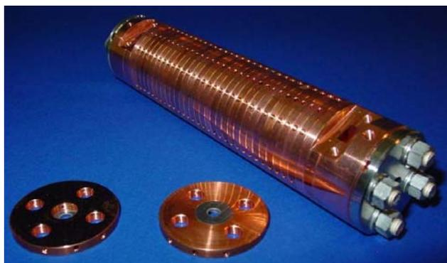
Figure 1: 30 GHz Molybdenum-iris structure.
