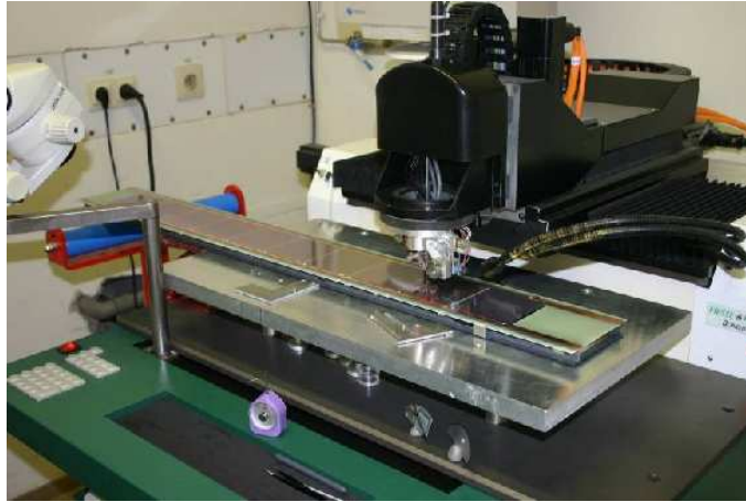
FIGURE 5.8. Construction of a Silicon ladder made of several Silicon sensors
