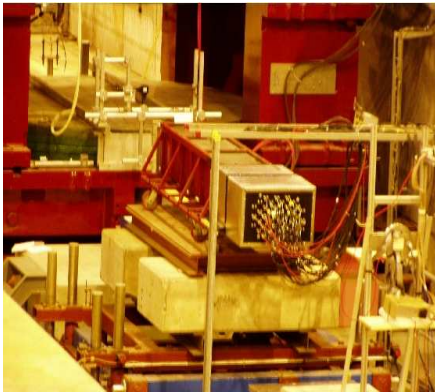
FIGURE 5.45. A DREAM module in the test-beam at CERN. The module is about 2 m in depth and 32 × 32 cm 2 in cross section.
