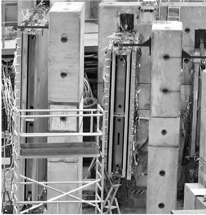
Fig. 3. Picture of the barrel tower consisting of two Inner, two Middle and two Outer MDT. The RPC attached to the Middle (center) and Outer (left) barrel MDT are also visible.
