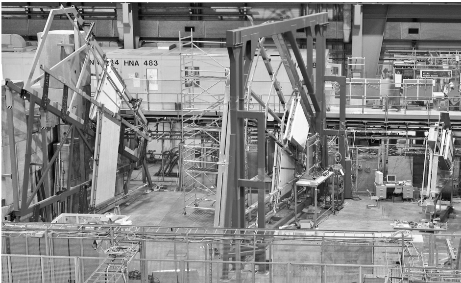
Fig. 2. Picture of the end-cap test stand with six MDT chambers and two TGC stations, taken in July 2003. From right to left: EOL, EML and EIL MDT chambers; the TGC doublets are close to the middle MDT station.
