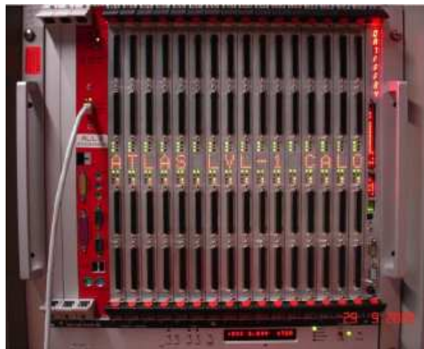
Fig. 2. A full crate of pre-production Pre-processor modules of the LVL1 calorimeter trigger. Most of the functionality of these modules is on replaceable Multi-Chip Modules (MCMs). These MCMs each contain a processing ASIC and four ADCs. All the MCMs (3000) are available, and production of the 124 Pre-processor modules is in full swing and expected to be finished by March 2007.
