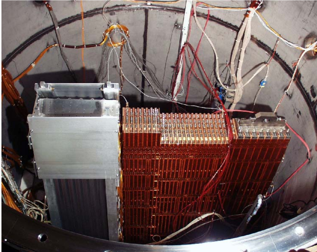
Figure 19: Top view of the first combined beam test showing in the cryostat (from left to right) the EMEC module with the pre-sampler, the three HEC front modules and the two HEC rear modules of reduced longitudinal size.
