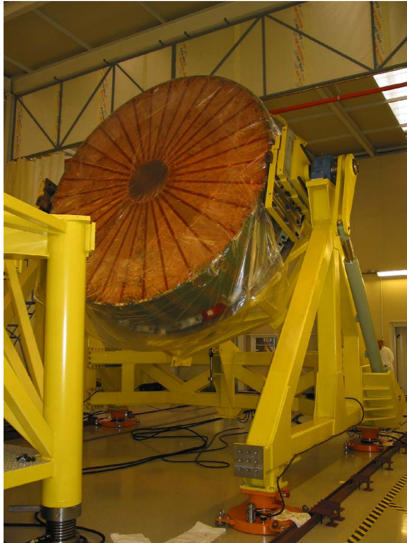
Figure 13: One of the two HEC1 wheels being rotated to the vertical orientation with the custom designed tooling after having being moved from the wheel assembly area. The wheel assembly stand can be seen on the left.
