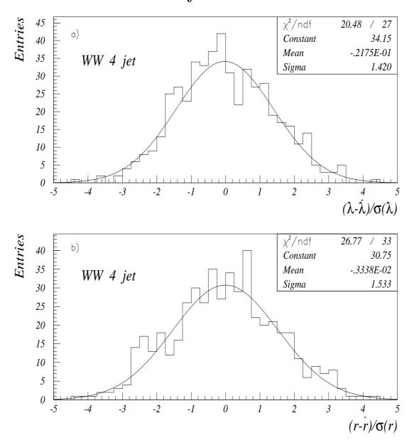
Figure 3: (a) Pull function for fitted parameter  $\lambda$  using a binned uncorelated least squares fit in the simulated samples. A gausian fit is supperimposed as a solid line. b) Same as (a) but for the parameter r.
