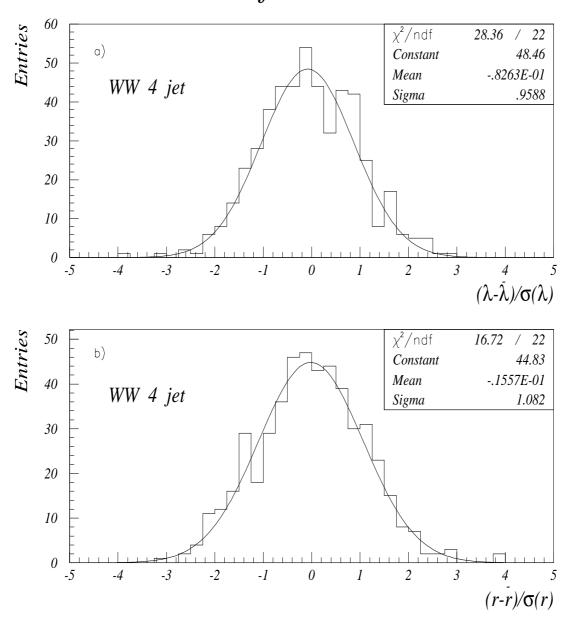
Figure 4: (a) Pull function for fitted parameter  $\lambda$  in the simulated samples using covariance matrix technique. A gausian fit is supperimposed as a solid line. b) Same as (a) but for the parameter r.
