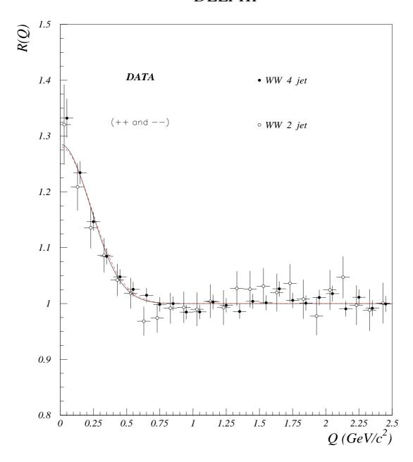
Figure 7: The measured correlation functions  $R_{2q}(Q)$  (open circles) and  $R_{4q}(Q)$  (closed circles) for like-sign pairs. The curves are the fit results using expression (3).
