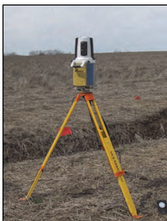
Fig. 1. Ground-based LiDAR utilized for gully formation and evolution studies in agricultural croplands.
