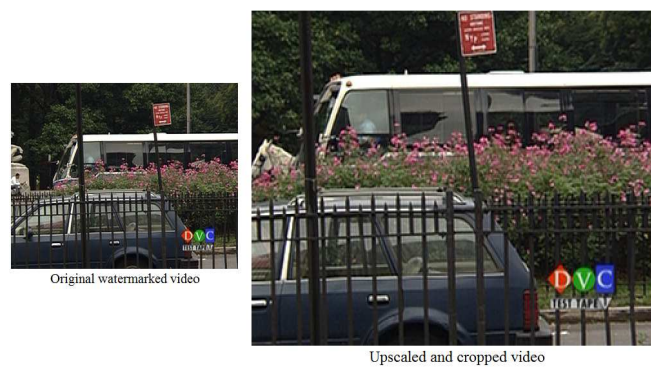
FIGURE 8. Example of upscaling by a factor of 2 with an uniform cropping of 10% along the edges.
