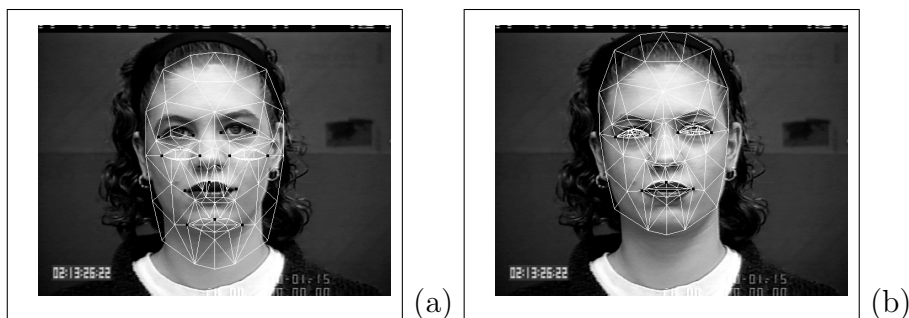
FIGURE 3. An example of mesh model fitting on a face image exploiting deformations. (a) The randomly initialized model on the face image, and the 7 manually defined correspondences between model nodes and face image features. (b) The model position after deformation.
