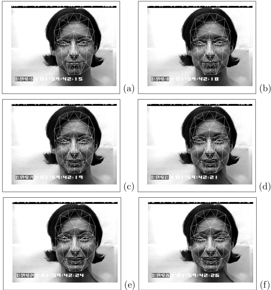
FIGURE 5. Model-based tracking in six uniformly sampled frames of a video sequence showing the full formation of a facial expression.
