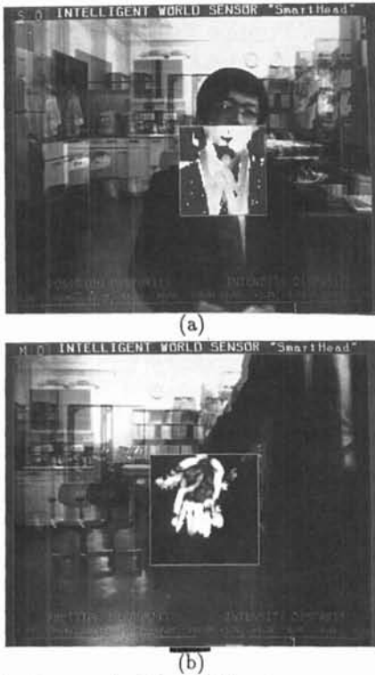
Figure 7. An example of the real-time shape reconstruction (a) and the image feature extraction (b). The central square of the monitor shows the processing region ( 64 \times 64 measuring points in 128 \times 128 area). In the region, a relative height map (a) with respect to the base plane and a strength map (b) of "ridgeness" feature is expressed by the degree of brightness.
