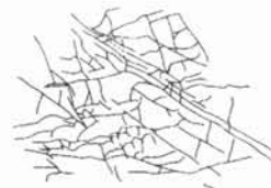
rock joints interpreted from rock surface image
