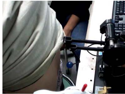
Figure 5 Measurement of the hardness and deformation of skin used PHANToM haptic device
