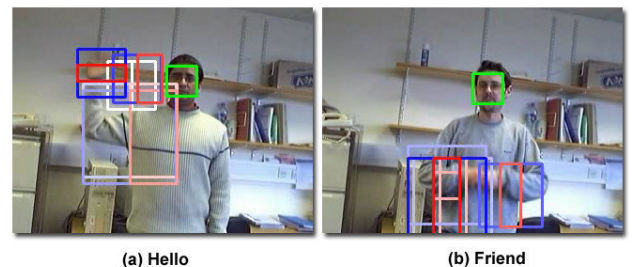
Figure 5: The first 20 classifiers chosen by the AdaBoost learning algorithm using T = 10 for the sign (a) 'Hello' which is a wave and (b) 'Friend' which is shaking hands with yourself.
