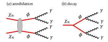
FIG. 4: Annihilating and decaying DDM model scenarios under consideration. The DDM components  $\chi_n$  annihilate or decay into the same intermediary particles  $\phi$ , which subsequently decay to two photons.
