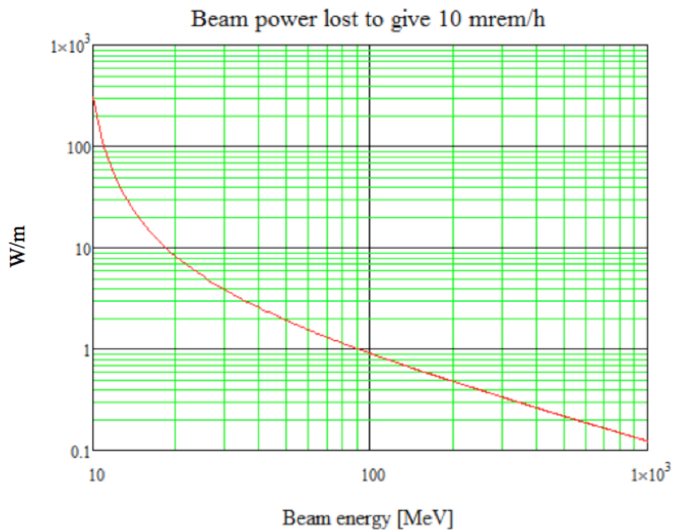
Fig. 7: Allowable beam power loss versus beam energy to produce an activation of 0.1 mSv/h (10 mrem/h) at 30 cm for the case of copper, after 4 h cool down.
