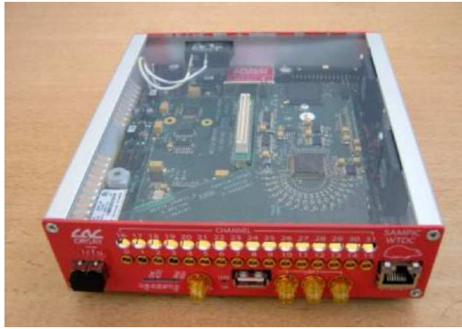
Figure 2: Picture of a 16-channel SAMPIC device.
