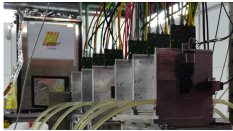
Figure 7: The telescope composed of six silicon planes.
