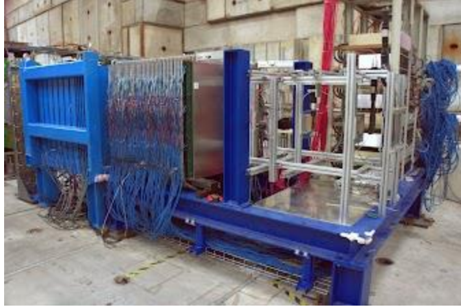
Figure 1. Photograph of the DHCAL setup at CERN showing the main stack with tungsten plates followed by the tail catcher with steel absorber plates.
