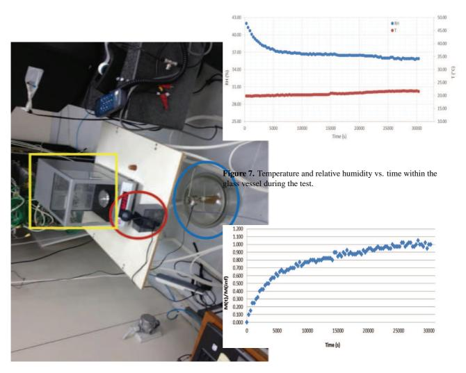
Figure 8. Humidity saturation trends in the GEM foil sample.
