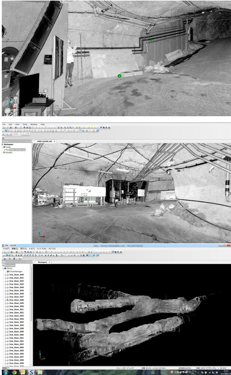
Figure 5.2: Top and middle: Two example scenes from the KamLAND tunnel as viewed in the SceneLT software. The green dots are targets used to align the coordinate systems of different sets of data. Bottom: Screen shot of Scene software viewing the point cloud from outside the tunnel from a vantage point somewhere in the rock.
