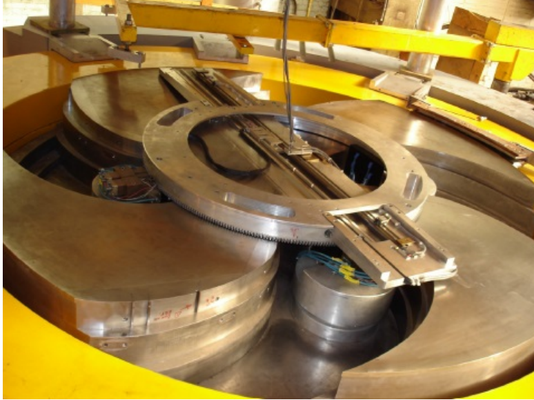
Figure 4.14: A mapping system installed in a similar cyclotron at IBA. (Image courtesy of IBA.)
