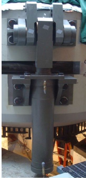
Figure 4.13: A hydraulic lifting system installed on a similar cyclotron.
