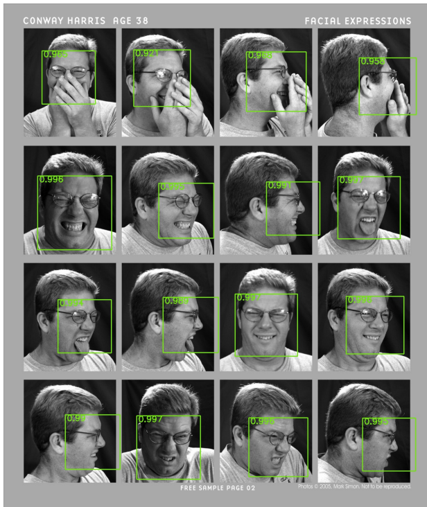
Figure 3: A set of faces with different out-of-plane rotations and occlusions. The figure also shows output of our proposed face detector after NMS along with the corresponding confidence score for each detection.
