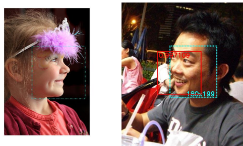
Figure 8: Annotation of a side face in left) training set and right) test set. The red bounding-box is the predicted bounding-box by our proposed detector. This detection is counted as a false positive as its IOU with ground truth is less than 50%.
