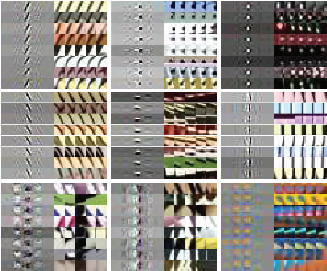
Figure 9. Deconvolutions of C3D conv2a feature maps. Each group is a C3D conv2a learned feature map. First two rows: the learned filters detect moving edges and blobs. The last row: the learned filters detect shot changes, edge orientation changes, and color changes. Best viewed in a color screen.
