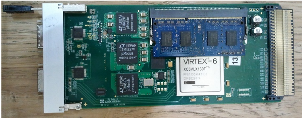
Figure 3. New Switch/Mux FPGA card
