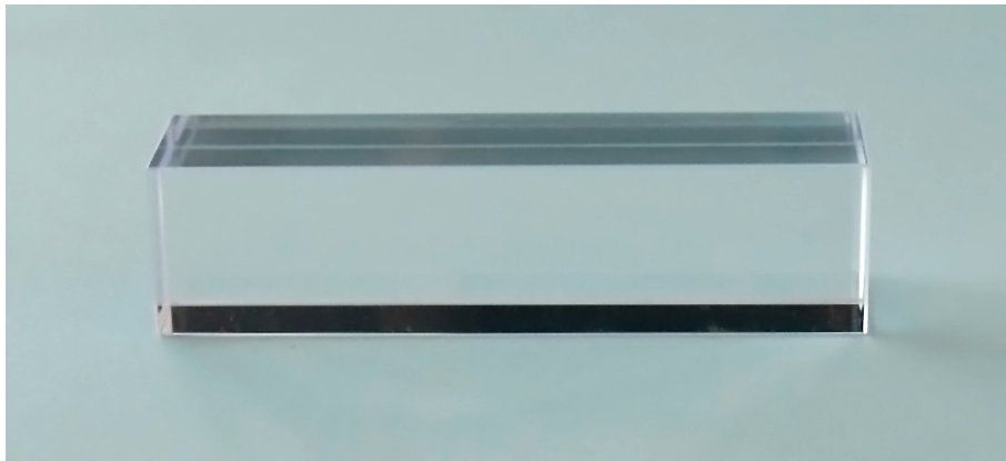
Figure 2: One of the tested LYSO samples, showing excellent mechanical processing and optical surface treatment.
