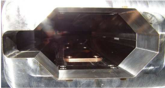
Fig. 5: Installed electrode in the dipole vacuum chamber.
