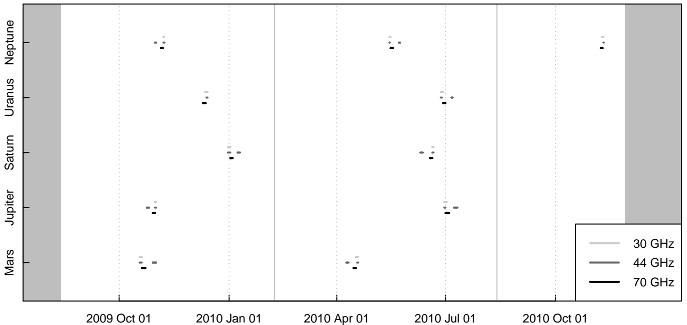
Fig. 22. Timeline of planet crossings. Each line shows the times when the planet fell within the beam of at least one of the radiometers at 30, 44, or 70 GHz. Gray bands at the edges mark the start of the survey and the end of the period considered in the 2013 data release. Vertical grey lines mark the separation between sky surveys.
