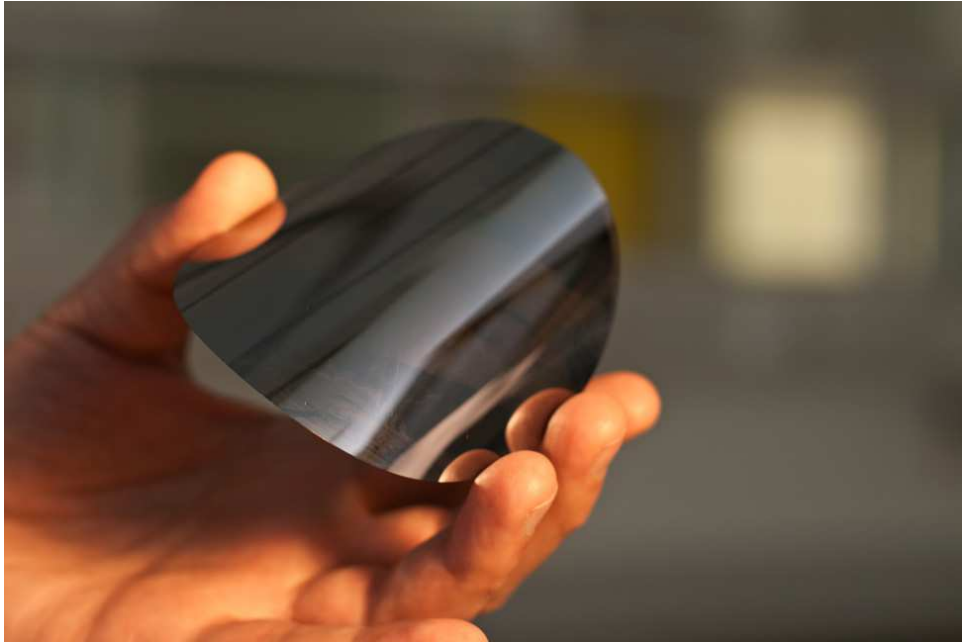
Figure 10.19: A 50 \mu\text{m} thin silicon wafer.
