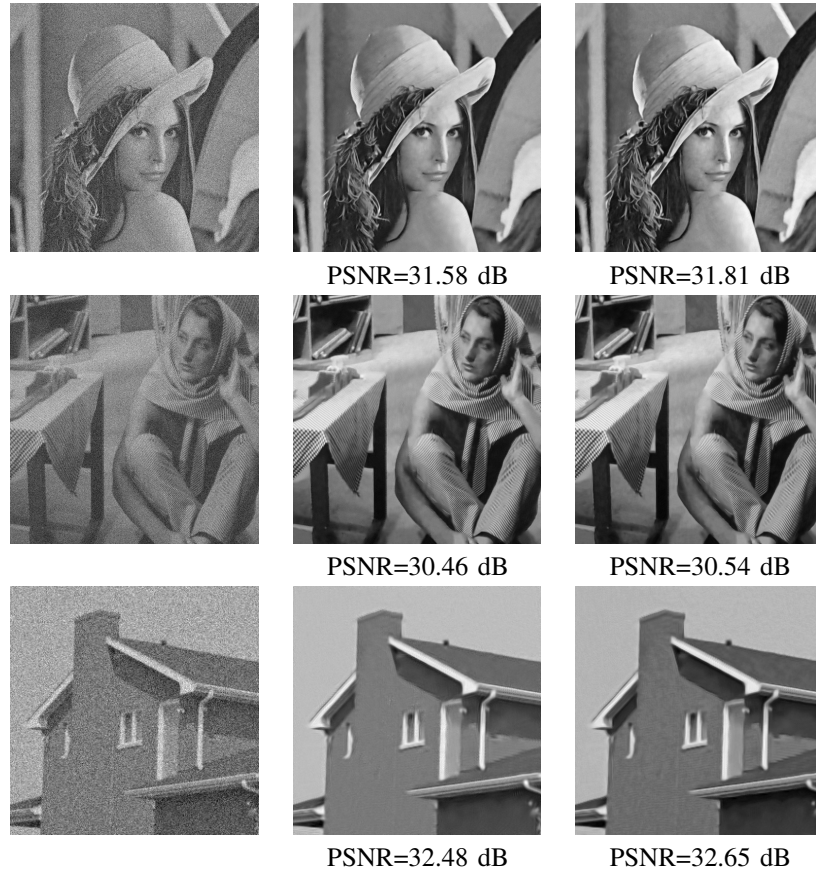
Fig. 6: Denoising results (PSNR) for the images Lena, Barbara and House ( \sigma = 25 , input PSNR=20.18 dB): Left column - noisy images, Center column - 1 iteration results, and Right column - 2 iterations results.
