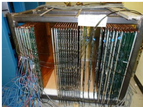
Figure 12: Photograph of completed cassettes undergoing cosmic ray testing.
