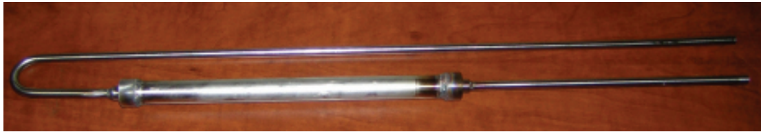
Figure 8.7: ^{222}\text{Rn} trap operated at SNO lab. The trap uses activated carbon spheres to slow transmission of radon atoms. The trap tested on removing Rn from Ar gas and operates at a -110^\circ\text{C} .
