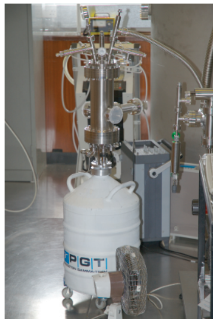
Figure 8.16: Photograph of the ZEPLIN III electron lifetime monitor positioned on the liquid nitrogen cryostat.
