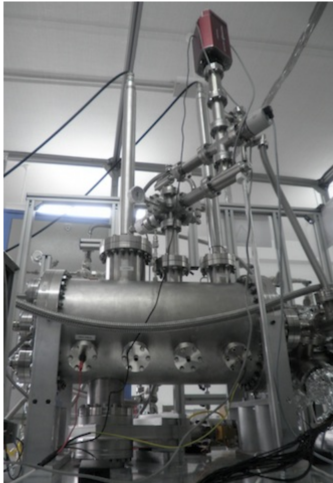
Figure 4.11: View of the NEXT1 pressure vessel. Also visible, the gas system, mass spectrometer and the long tubes to pass the high voltage.
