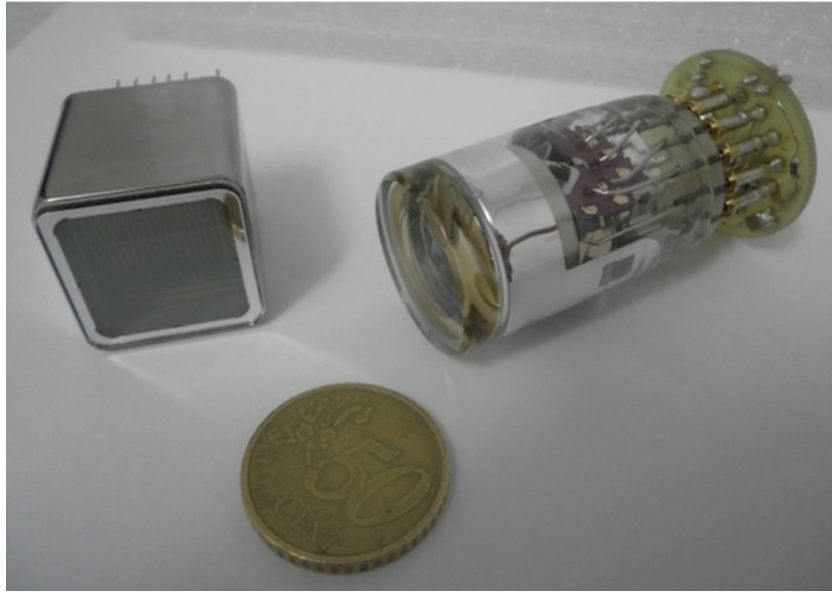
Figure 3.1: On the left, the Hamamatsu R8520-406 PMT. This is a radiopure PMT, sensitive to VUV, that can take up to 5 bar pressure. On the right, the PMT used in the NEXT-1 prototypes, model R7378A. This phototube is also sensitive to VUV and can resist pressure up to 20 bar, but is not radiopure.
