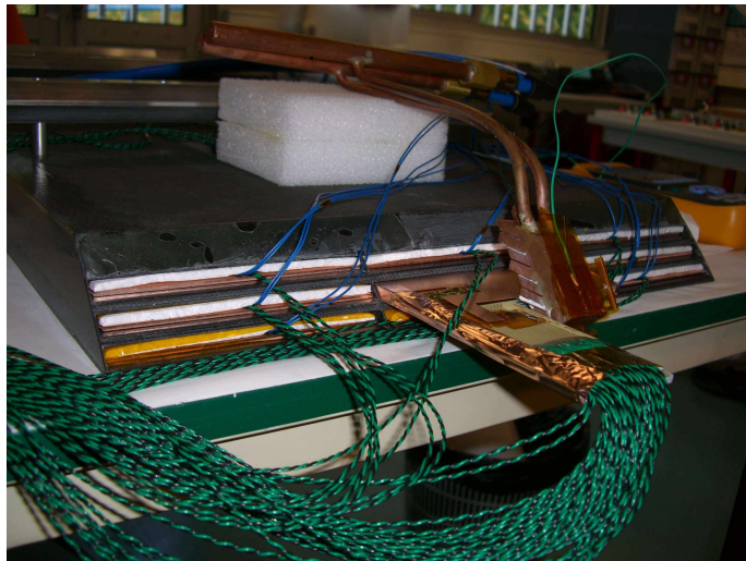
Figure 10. Cooling tests using the demonstrator module. The ends of the nine thermal slabs are visible at the end of the mechanical structure, as is the copper heat exchanger connected to the slabs' thermal drain.
