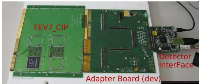
Figure 7. DAQ test hardware: prototype ASU - adapter board - Detector InterFace card.
