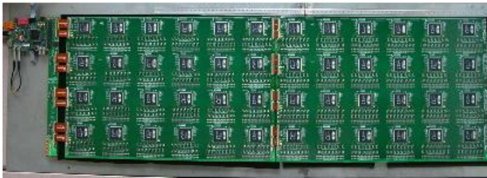
Figure 43. Photograph of 2 ASUs of 48 \times 32 \text{ cm}^2 with 24 HARDROC2 chips chained with flexible cables, readout boards (DIF and inter-DIF) appear in the top left corner.
