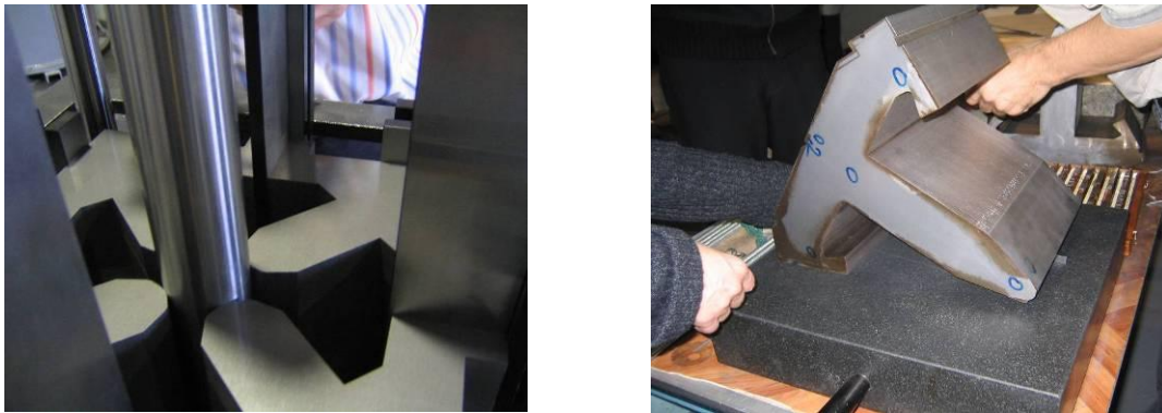
Fig. 20: Left: Stacking fixture of laminations for ALBA Storage Ring quadrupole. Right: Mechanical test of finished yoke for ALBA Storage Ring sextupole magnet.
