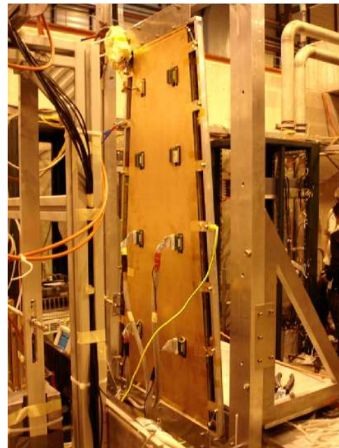
Fig. 11. GE1/1 Installed at the Test Beam.
