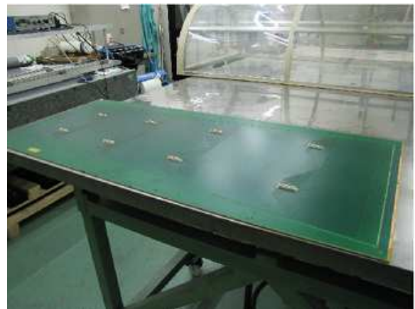
Fig. 7. GE1/1 PCB readout plane.
