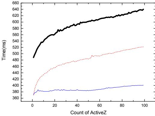
Fig. 13 Improvement at retrieving pair production cross data due to the design based on templates (dashed red curve) and on the use of `unordered_map` along with the new design (thin blue curve), with respect to the original classes (thick black curve).
