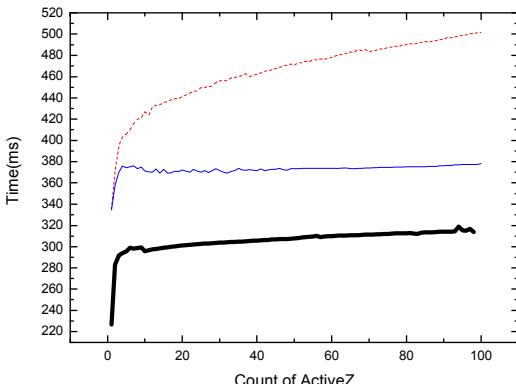
Fig. 15 Performance overhead due to using `unordered_map` (thin blue line) or a map (red line) in the new design scheme, with respect to the original design using a STL vector and loading all 100 data sets of Rayleigh form factors (thick black line).
