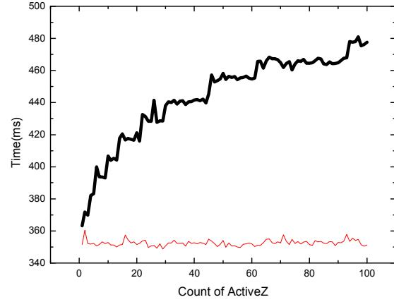
Fig. 7 The retrieval of pair production cross section data as a function of the number of instantiated elements: current Geant4 implementation (thick black curve) using the `map` STL container and implementation using `unordered_map`, which is foreseen for inclusion in the forthcoming edition of the C++ language.
