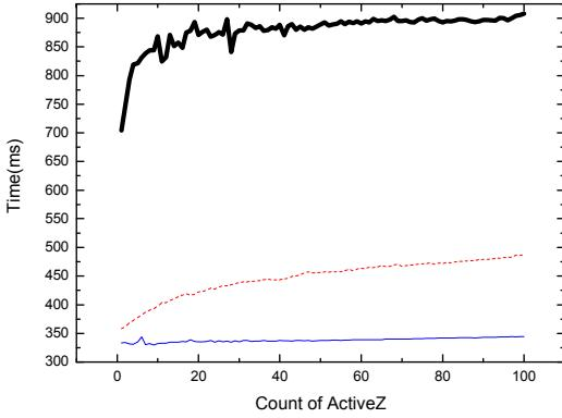
Fig. 14 Improvement at retrieving Bremsstrahlung spectrum data due to the design based on templates (dashed red curve) and on the use of `unordered_map` along with the new design (thin blue curve), with respect to the original classes (thick black curve).
