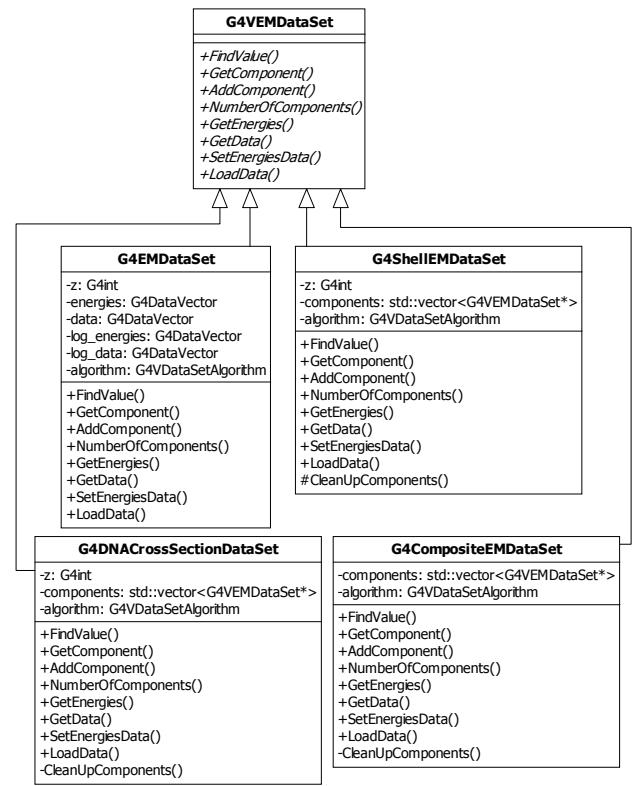
Fig. 1 UML class diagram illustrating basic data management.
