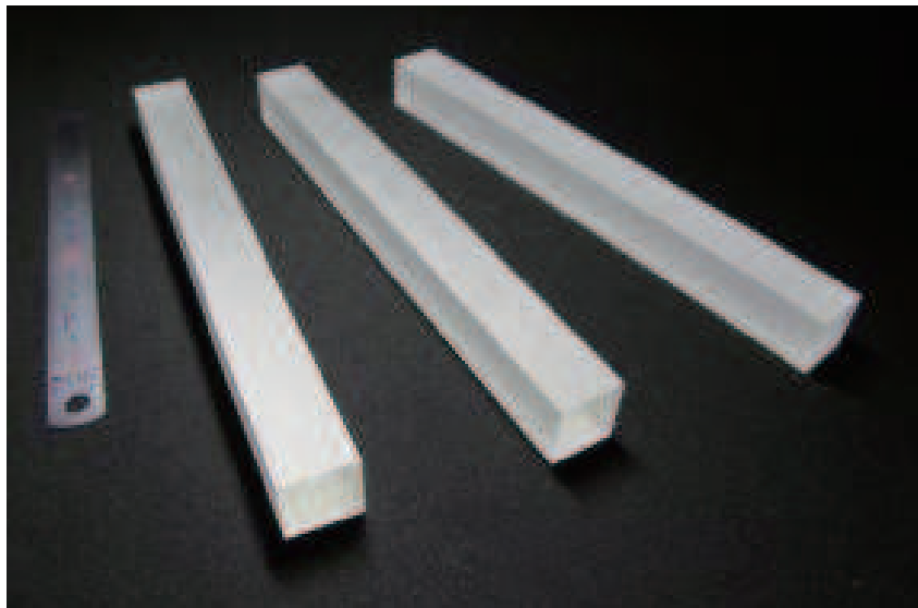
Figure 9.24: The \text{Bi}_4\text{Si}_3\text{O}_{12} (BSO) crystals with 2 \times 2 \times 20 \text{ cm}^3 dimensions produced by Oxide.
