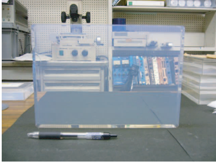
Figure 8.8: A large-size ( 180 \times 260 \times 20 \text{ mm}^3 ) aerogel tile.
