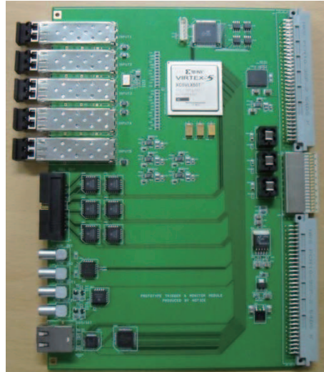
Figure 12.16: A photograph of the 6U-VME TMM pre-prototype board. The final design will be implemented on a 9U-VME board to accommodate the input/output connectors.
