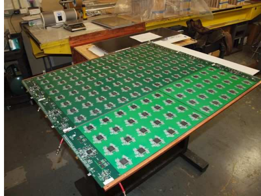
Figure 5: Photograph of a detector layer with six front-end boards.
