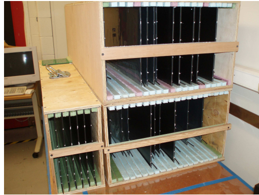
Figure 2: Photograph of completed RPCs (some with the high voltage connector not yet installed).
