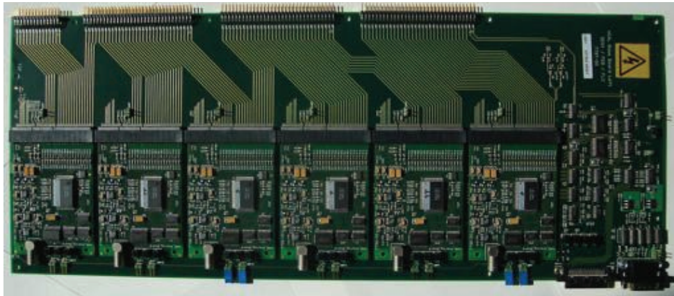
Figure 18. The VFE AHCAL base board with six mezzanine boards. The connection to the SiPMs is via coaxial cables.
