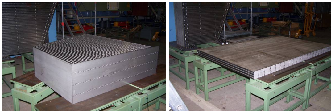
Figure 26: The two vertical (left) and the horizontal (right) mechanical structures for the technical HCAL prototype.
