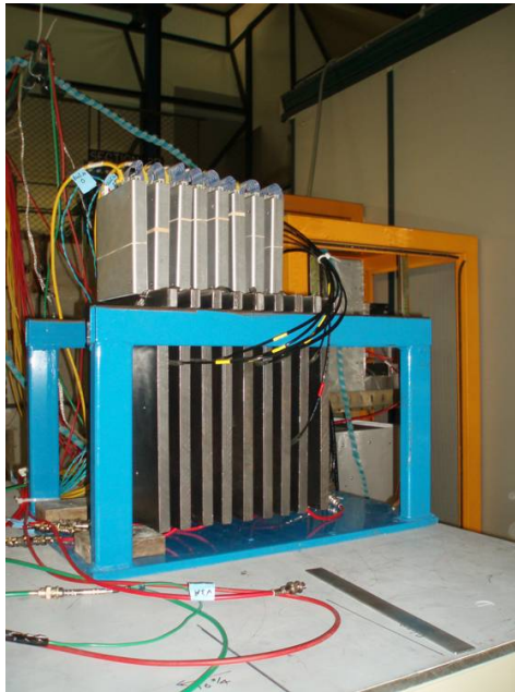
Figure 28: Photograph of the Vertical Slice Test in the FNAL test beam.
