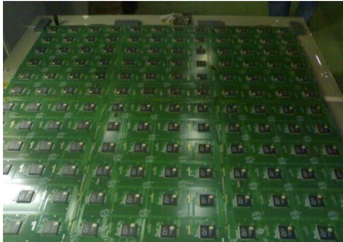
Figure 34: Layout of HARDROC2, view of the chip packaged in TQFP160 and square meter prototype of RPC DHCAL with 144 HARDROC.
